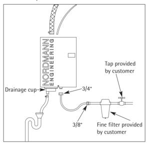
In any case the water feed pipes must be flushed thoroughly before connecting them to the humidifier. You should use copper piping only.
